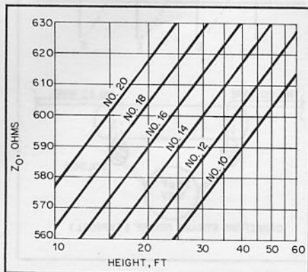
Fig 3— Z_0 versus height and wire size. Z_0 = 138 \log(4h/d)
